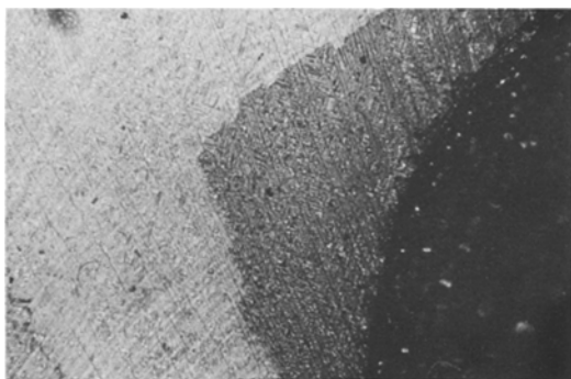
Figure 3 Photograph of MgO surface after an Al drop had been in contact with the surface for 1 h at 1300 K. The foot of the drop is the circular section on the right. Away from the Al drop the MgO surface has been etched. The intermediate zone displays the diffusion effects described in the text ( \times 45 ).
